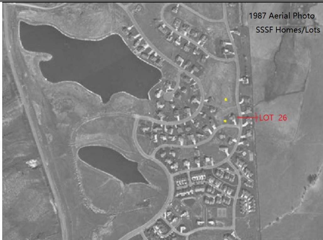
This 1987 Aerial Photograph above shows (between the two yellow dots) a creek existed between Lots 26 and 27. Neighbors remember traversing its small bridge. Just how filling-to-extinction, the small creek on Lot 27, affected subsurface flow is speculation at this point.
